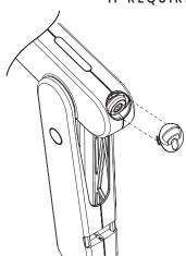
If required, manual adjustment feature can be disabled by fitting a cover.
